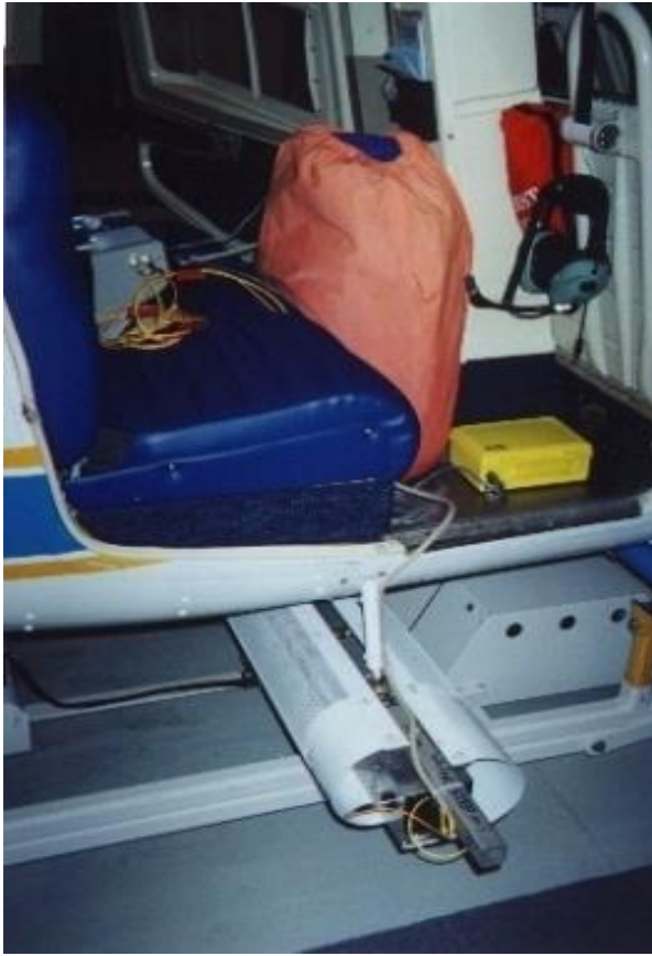
GasFinderAB mounted in helicopter cabin (left) and multiple pass cell mounted under cabin (right).
