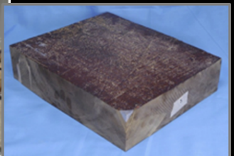
3-D, multi-layer preform weaving technology for thermal protection
